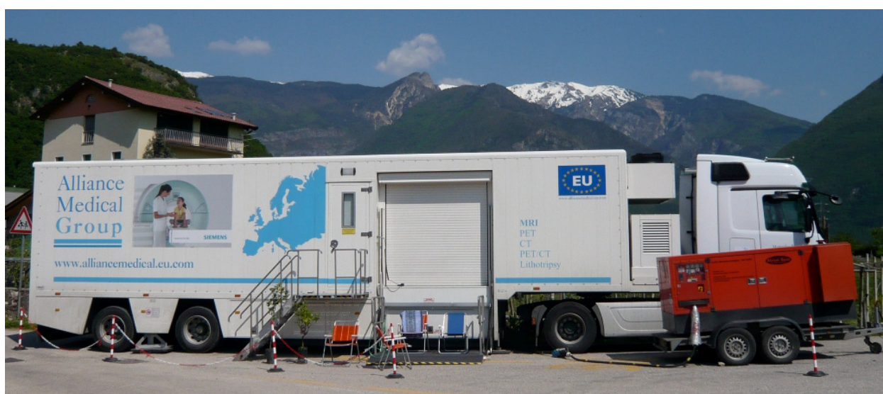
Figure 2 Truck trailer with mobile MRI and external generator in working position.
